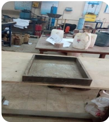
Figure (6) The wheel tracking test specimen
