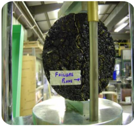
Fig. (2) Schematic of Indirect tensile test setup
