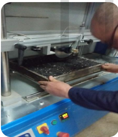
Figure (7) Operation the wheel tracking test device
